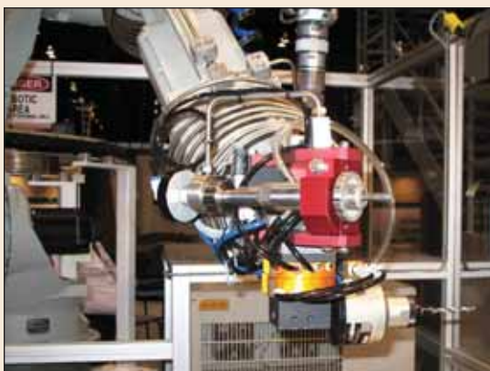
QC-41 with G19 electrical module
