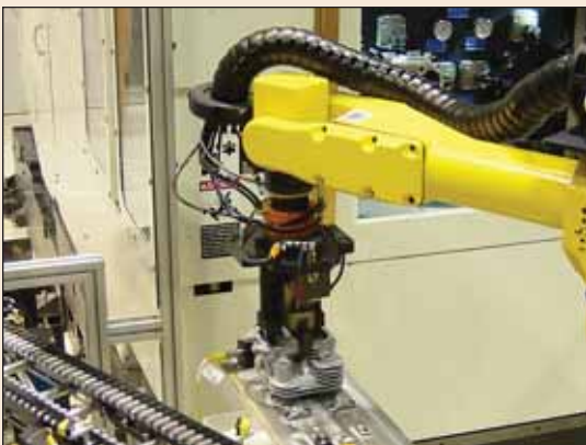
QC-60 with K26 electrical module
