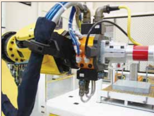
QC-150 with T19 electrical module
