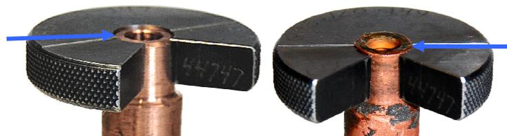
**Incorrect taper** – the adapter does not measure within the allowable engagement range
